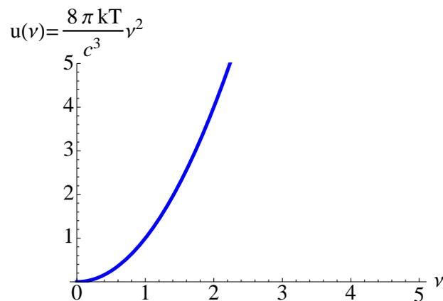
As Rayleigh-Jeans law suggests, the energy density increases with increase in frequency. But as observed from experiments, the energy density decreases exponentially at large frequency or at small wavelength (thus the name Ultraviolet!). The failure of the Rayleigh-Jeans law at large frequency is known as Ultraviolet Catastrophe.
